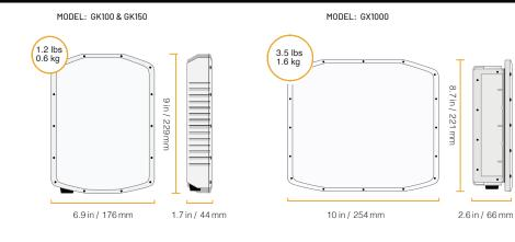
The GK and the GX series radars use an Active Power over Ethernet connection, making installation easier and more cost effective while maintaining high performance when tracking threats.
